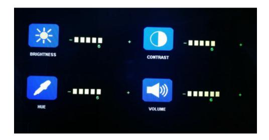
Press + or - to select BRIGHTNESS, CONTRAST, HUE OR VOLUME and then press AV to enter the setting. Once the icons turn red they can be adjusted. Press + or - to adjust values up or down. Press M to exit the menu. Press M again to return to the main menu.
