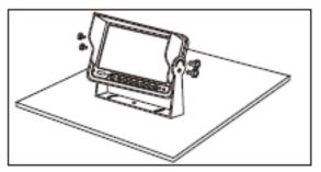
The monitor can be adjusted 30° forwards and backwards. Select the desired angle for optimal viewing.
