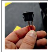
Reconnect switch to crimp terminals and locate a suitable place for mounting the switch, you will need to drill a 20mm hole to facilitate the switch. Suggested location shown (side of the steering wheel).
