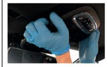
Pull the centre of the interior light panel down and uplug and remove.
