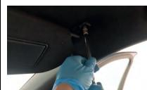
Undo the 2x 7mm bolts and uplug the sunvisors.
