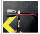
Remove Switch from the crimp terminals and cut of the lamp connector from the wiring harness.
