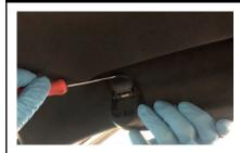
Using a small flat blade screwdriver, pull down the bolt cover and undo the 2x 8mm bolts.
