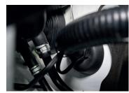
Route the lamp wiring through the factory grommet, make sure a drip loop is made with the cable to prevent water ingress. The cable will fall into the left footwell.
