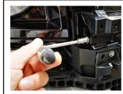
Install the outboard brackets as shown (1x either side).
