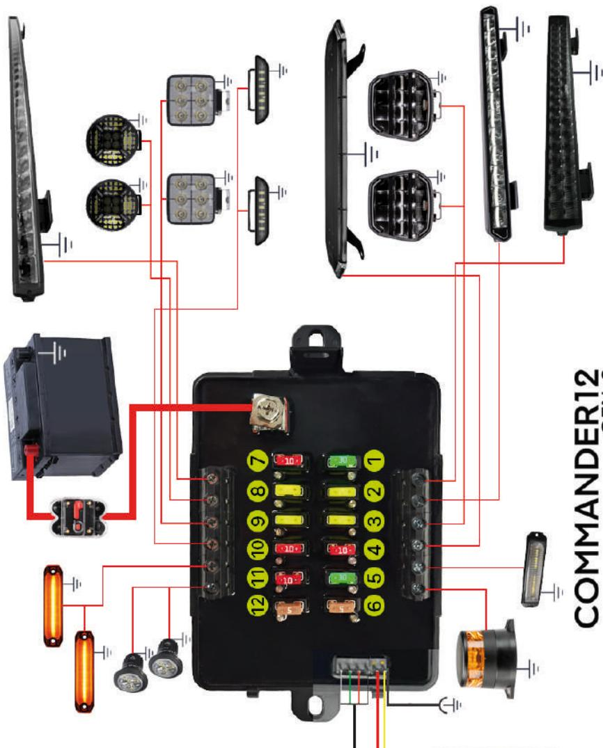
The small **red** wire connects to an accessory circuit in the vehicle. This configuration allows the outputs to be disabled when the key accessory is off.
