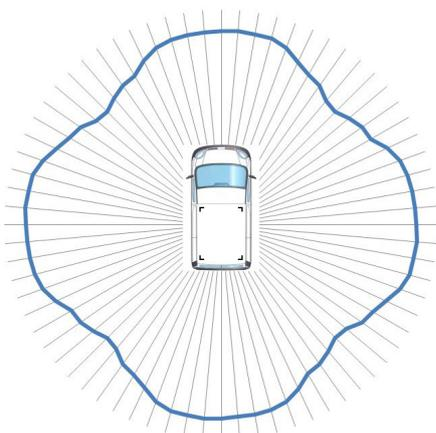
4 Corner Module LEDs fitted on the corners of a vehicle produce a strong homogeneous 360° warning signal as shown in the diagram.
